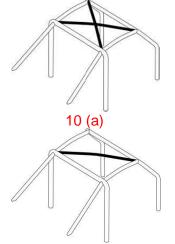
10(b) Bar may be fitted in either orientation.
